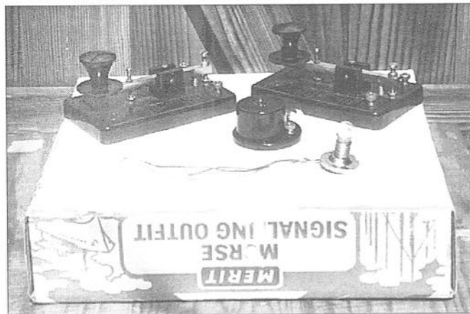
Merit Morse Signalling Outfit, comprising two keys, buzzer, lamp, and two coils of wire. Later version of No.350 set
