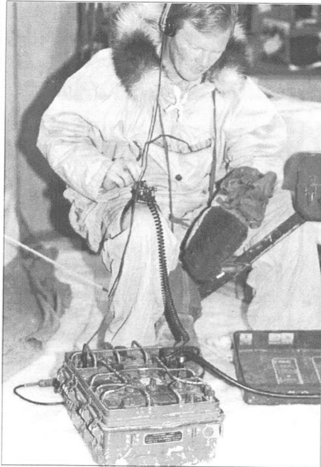
Melbourne 1997. Mawson 1985 Radio Technical Officer David Jewell demonstrating a still functioning Angry-9 field transceiver with knee-mounted key.
