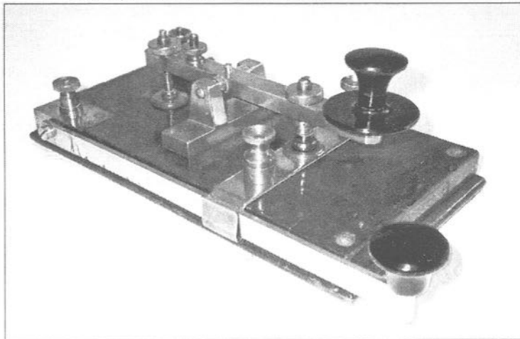
Jack Barker's Marconi Manipulating Key, circa 1912 – now fully restored except for the nameplate. A massive but beautifully balanced key.
