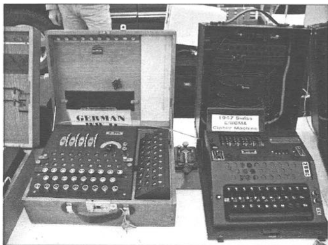
The model "K" Enigma with remote light panel, a typical German Naval telegraph key made by Junker, and the Swiss NEMA with remote light panel.
