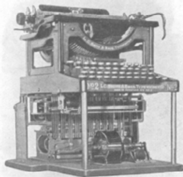
Burlingame Telegraphing Apparatus Attached To an "L. C. Smith" Typewriter
