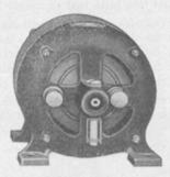
Induction motors operate on alternating current and are characterized by running at practically uniform speed regardless of load. They are extremely reliable on account of the absence of brushes, commutators, etc., and are to be recommended wherever alternating current is available and variable speed is not essential or can be secured by a change in pulleys.
