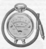
These meters provide an inexpensive and convenient method of testing dry batteries, storage batteries, low voltage lighting systems, and not only indicate volts and amperes but also show the polarity and avoid the necessity of carrying a separate polarity indicator. They are furnished with black letters on a white dial. Cat. No. H. 020. Ammeter 1\frac{1}{4}" face, reading 0-40 amperes. Price \$1.00 Cat. No. H. 021. Voltammeter 1\frac{1}{4}" face, reading 0-10 volts, 0-30
