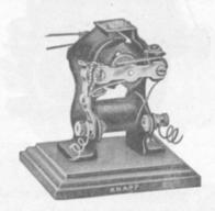
This little motor will run on one dry cell, is 31 inches high, finished in black enamel with nickel plated trimmings and the binding posts and switch are mounted on the field to avoid disturbing connections when using the motor without the base. The 1/8 inch shaft is fitted with a pulley for running mechanical toys, etc. Shipping weight 1 lb.
