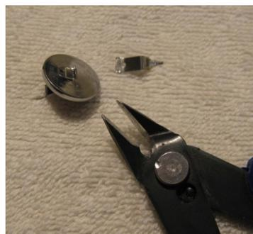
11. Flatten the solder tabs, and lightly tin them with solder.
